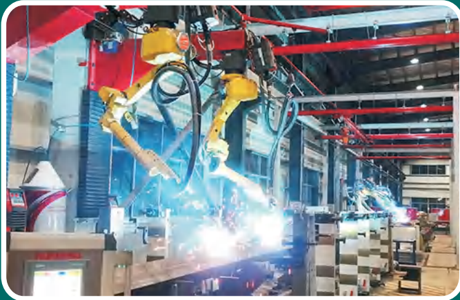
Truss Automatic Welding Production Line
